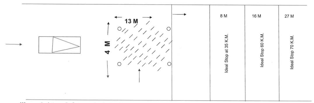
When passing between the first cones, the clutch pedal must be activated and when passing the next cones, the brake pedal must be activated.
